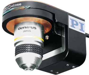
Instead of moving the sample, it is also possible to move the objective. The P-725 PIFOC® Objective Scanner offers travel ranges over 400 µm with nanometer resolution and response times in the millisecond range
