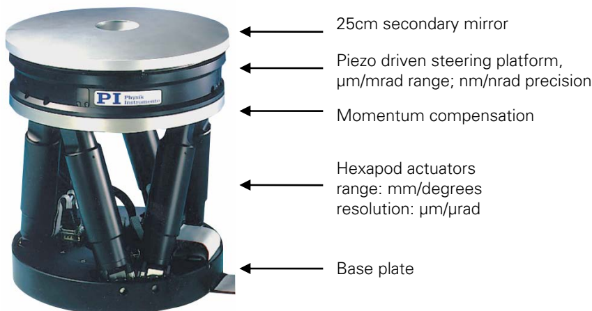
Example of a combined high-speed piezo tip/tilt platform with a long range, low-speed 6-axis hexapod alignment system
