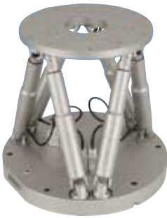
M-850 High Load 6-Axis-Alignment System; Works in Any Orientation; No Moving Cables; 200 kg Load Capacity (Vertical); Heavy-Duty, Ultra-High-Resolution Bearings for 24/7 Applications; Repeatability to \pm 1 \mu\text{m} ; Encoder Resolution to 0.005 \mu\text{m} ; MTBF 20,000 h
