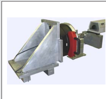
Tzec Maun Telescope Secondary Tip/Tilt Mirror \varnothing 290 \text{ mm} , 100 \mu\text{rad} Tip/Tilt, 50 Hz Bandwidth 100 nrad Resolution, > 650 \text{ Hz} Fres Rise time 3 ms (small angle), 5 ms (large)
