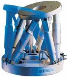
M-850 High Load 6-Axis-Alignment System; Works in Any Orientation; No Moving Cables; 200 kg Load Capacity (Vertical); Heavy-Duty, Ultra-High-Resolution Bearings for 24/7 Applications; Repeatability to \pm 1 \mu\text{m} ; Encoder Resolution to 0.005 \mu\text{m} ; MTBF 20,000 h
