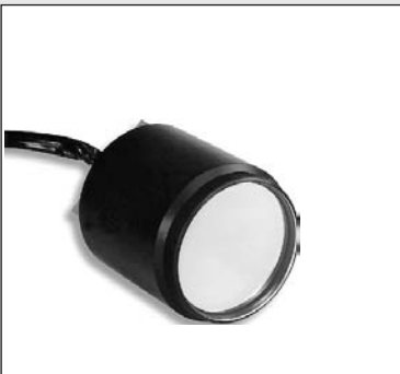
Active secondary tip/tilt mirror for the 2.2 m ESO (European Southern Observatory) telescope in La Silla, Chile. Mirror diameter: 100 mm Tip/tilt range: \pm 400 \mu\text{rad} Resonant frequency: 900 Hz
