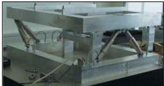
Large custom Hexapod with a positioning frame measuring some 1.0 x 1.5 meters.
