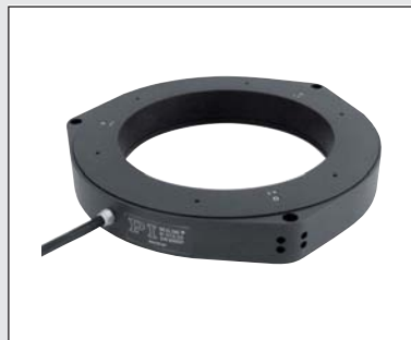
PiezoWalk® Tripod: Z/Tip/Tilt Stage Ø300 mm, 200 N load capacity, 1.3 mm piston, 10 mrad tilt range
