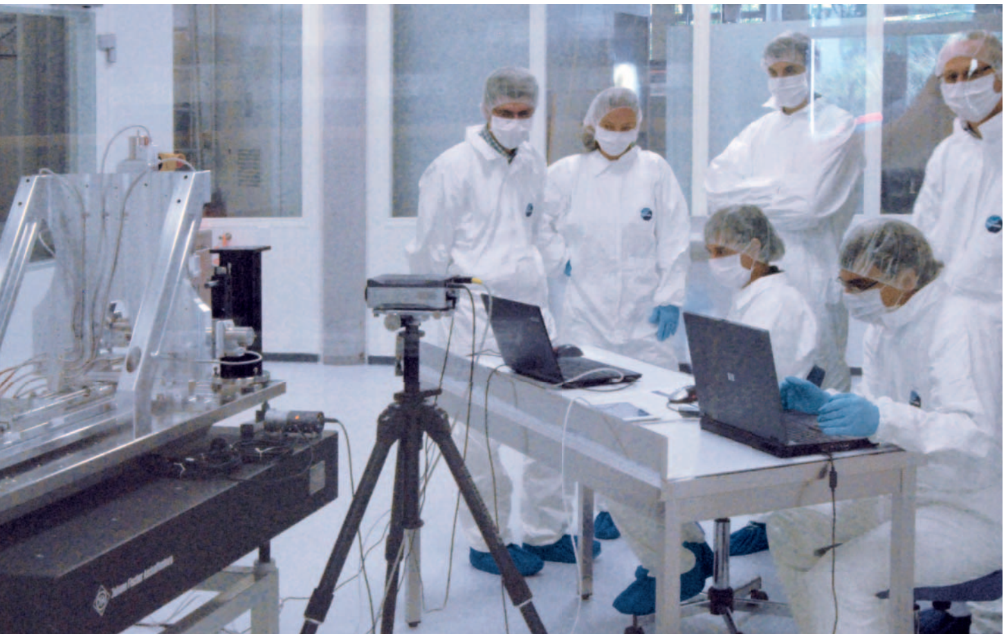
Commissioning of a vacuum-compatible multi-axis system and qualification on site (Image: HZG / DESY)
