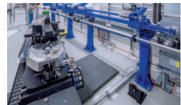
The whole assembly is moved to the parking position outside the beam on air bearings (Image: PI / HZG)
