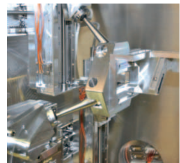
SpaceFAB advantage: A long stroke in X allows to place the platform with the lens outside of the beam
