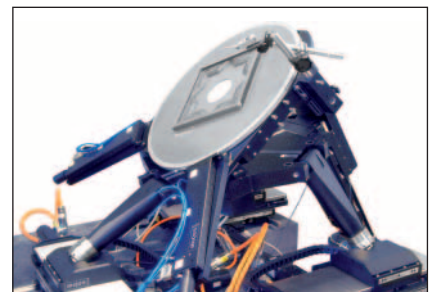
10-axis sample positioner, inclined 45° to the beam
