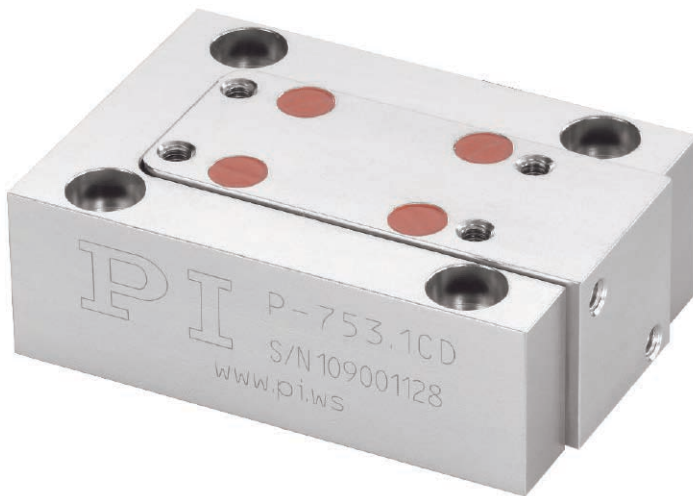
P-753.1, dimensions in mm. Max. torque at M2.5 threads: 0.3 Nm.
