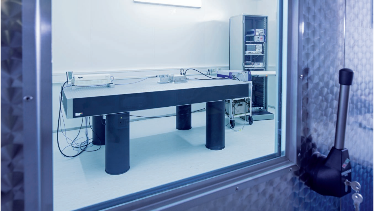
View of a nanometrology laboratory with six-fold insulation. Qualifying is done here fully automatically under controlled ambient conditions
