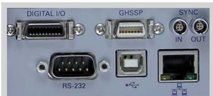
PI controllers are available with a number of different interfaces for highest flexibility. In addition to the modern Ethernet (TCP/IP) and USB, many industrial customers still appreciate the robust RS-232 protocol
