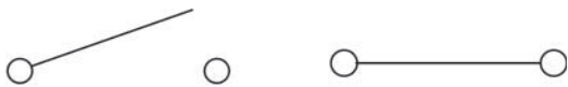
Air pressure below the threshold value, pressure switch opened (left). Air pressure above the threshold value, pressure switch closed (right).
