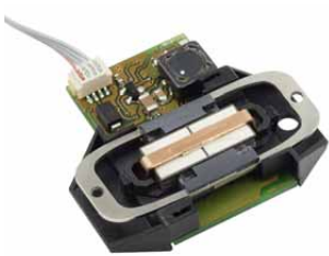
Sub-thumb-sized: a U-155 integrated piezo linearmotor for micro mechanical systems, with control electronics. The silver spring doubles as a moving carriage.
