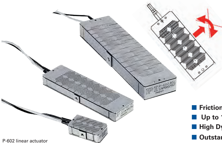
P-602 linear actuator family featuring travel ranges of 100, 500, and 1000 \mu\text{m} (from left to right). Flexure guides provide straight motion without tip and minimum tilt
