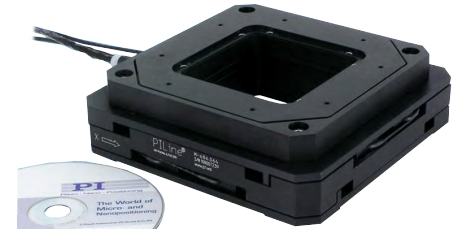
M-686 open-frame stage with P-541.2DD piezo scanner on top, providing a resolution of 0.1 nm and a scanning range of 30 x 30 \mu\text{m} . The system height of the combination with the P-541 XY (or Z) piezo scanner is only 48 mm
