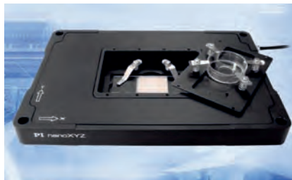
The P-545 piezo stage provides 200 µm travel per axis with sub-nanometer resolution. PI nano™ features a larger aperture for 1x3" slides.
