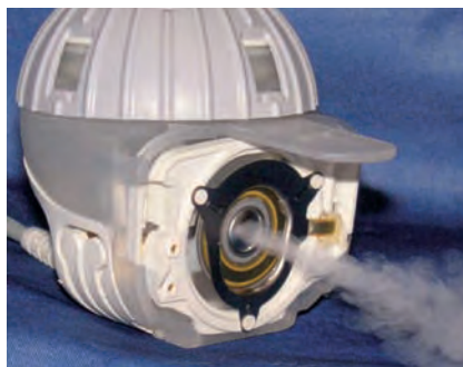
An annular piezo disk serves as an ultrasonic transducer to produce the aerosol in the atomizer head of the eFlow® rapid Electronic Nebulizer series. (source: Pari Pharma GmbH)
