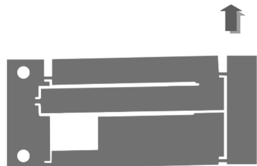
The flexure guiding system prevents tip and tilt at the drive head!
